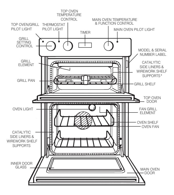
NEVER line the shelves, floor or sides of the oven or grill with aluminium foil as overheating and damage may result.
